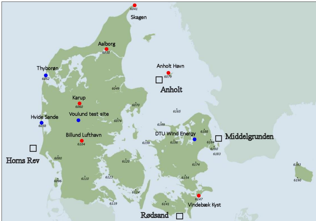
Figure 11: Location of DMI weather stations (dots with numbers), disdrometers (blue dots) and sections for evaluation of radar now-casting near selected wind farms (black boxes). Wind farm names are shown, but not the exact location.
