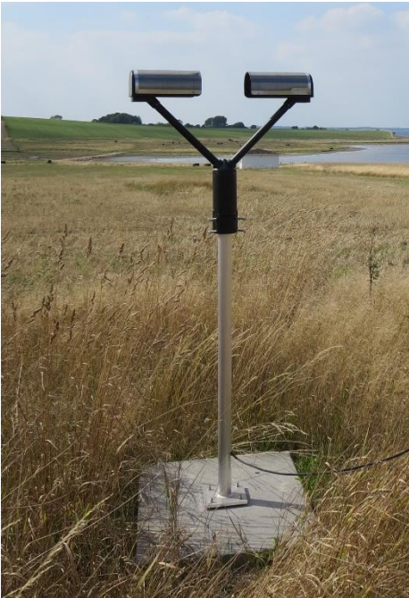
Figure 4: Disdrometer installation at DTU Risø campus at the true wind site (RTW)
