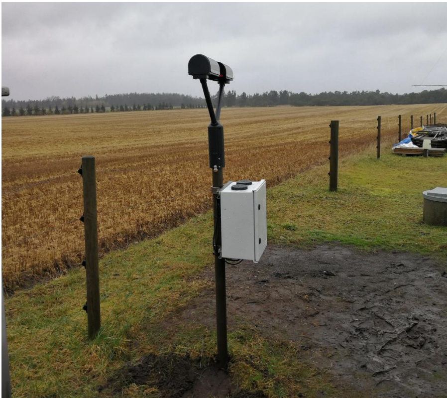
Figure 8: Disdrometer installation in Voulund - DVO
