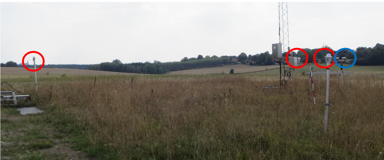
Figure 10: Three WS100 radars (WS-RTW) – indicated by red circles - and disdrometer (RTW) – indicated by a blue circle - at the true wind site within short distance
