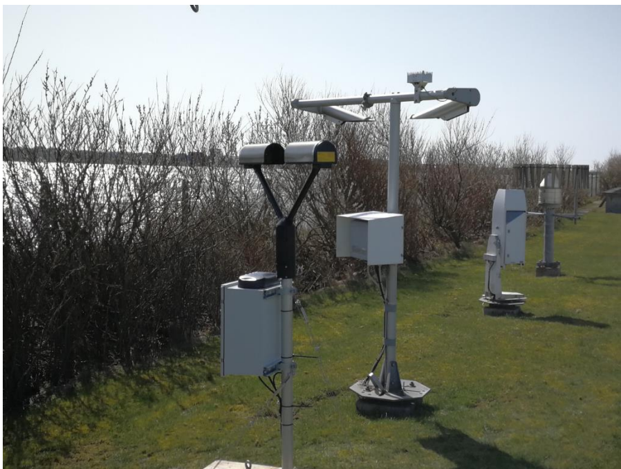
Figure 6: Disdrometer installation in Hvide Sande – DHS - next to the Weather Sensor (Vaisala FD12P)
