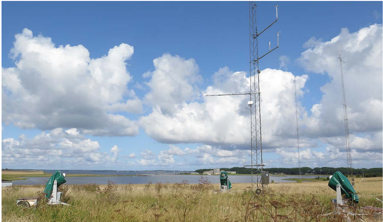
Figure 6. The test site at DTU Risø Campus with three WindScanner lidars measuring in the vicinity of the Parsivel 2 disdrometer and the three WS100 radar-based disdrometers.
