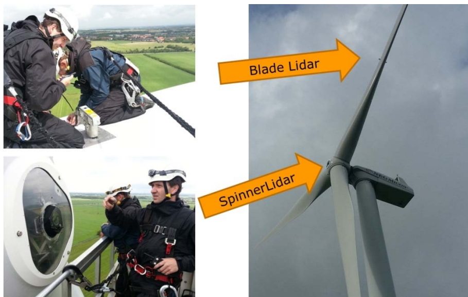
Figure 2. Turbine-mounted SpinnerLidar and blade-mounted Lidics developed in previous DTU-lead projects. The novel precipitation detection lidars are utilizing existing hardware but with novel processing algorithms.
