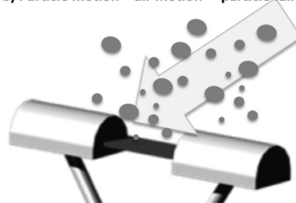
b) Particle motion = air motion + particle fall velocity
