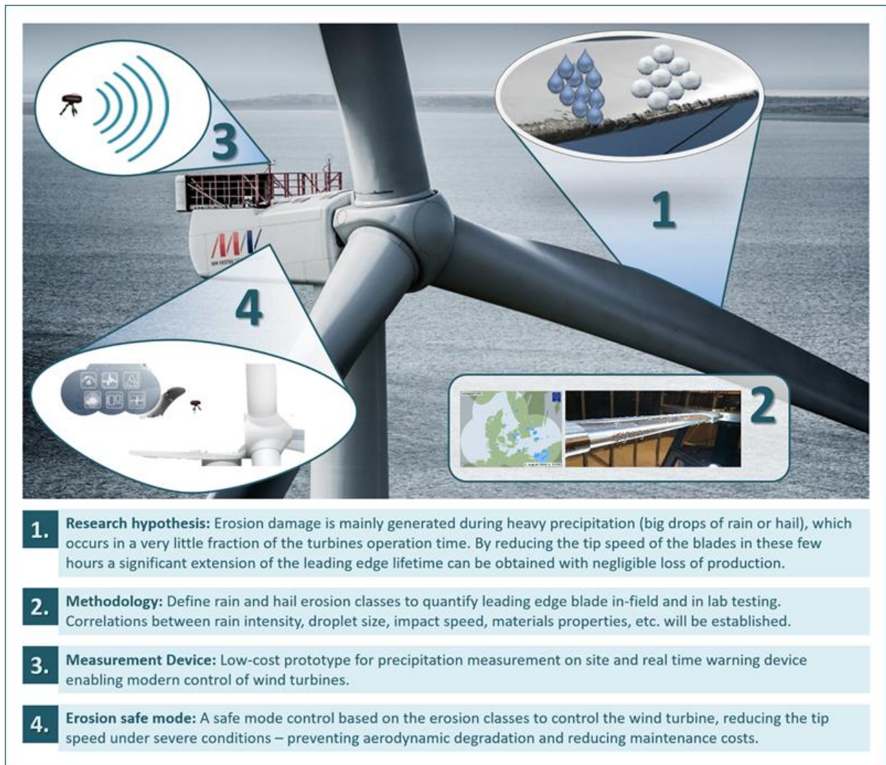
Figure 1. Sketch of the research hypothesis in the EROSION project.
