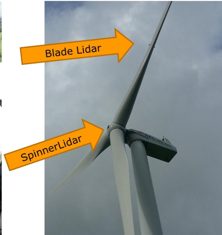
Turbine-mounted SpinnerLidar and blade-mounted Lidars developed in a previous DTU-lead project. The novel precipitation detection lidars are utilizing existing hardware but with novel processing algorithms.
