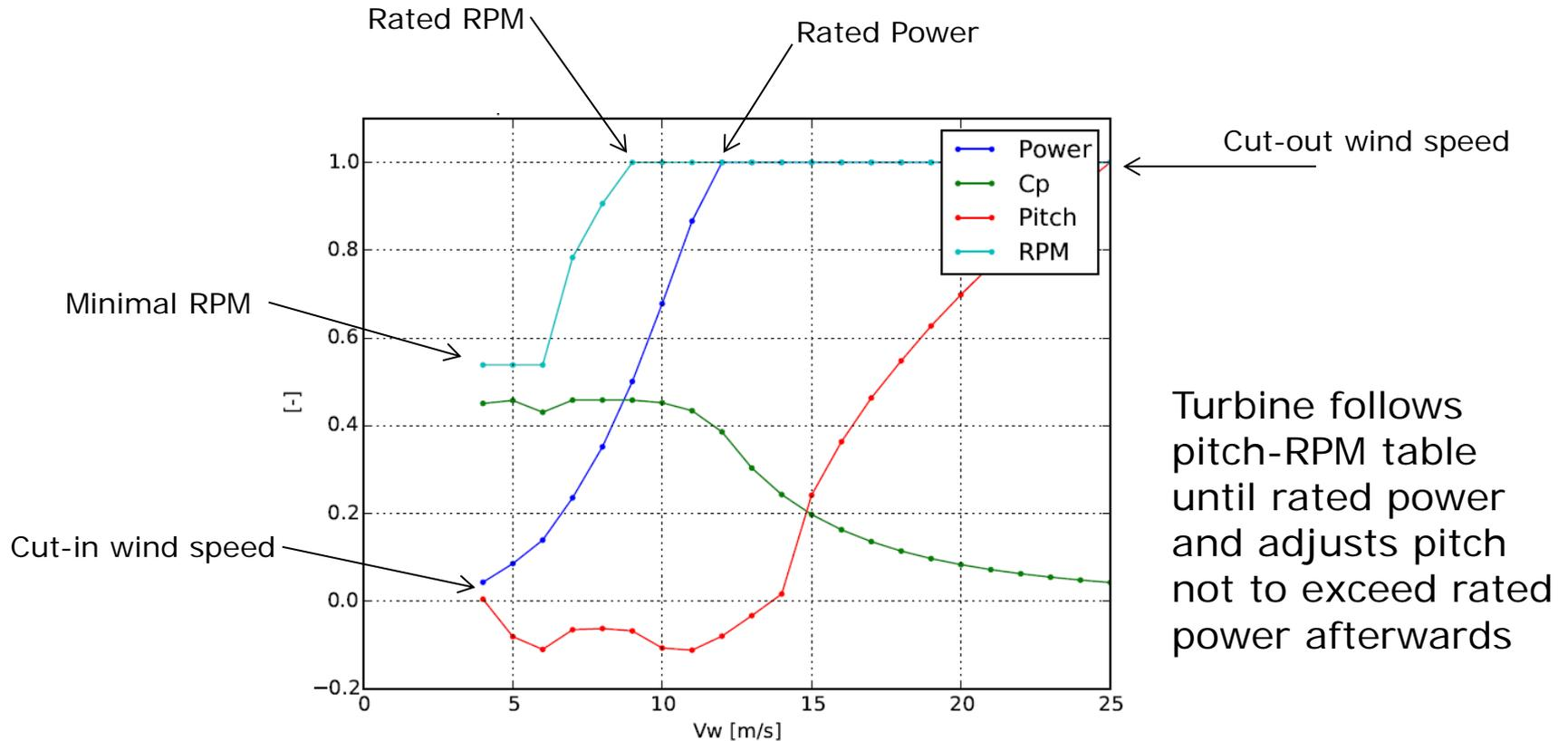
Turbine follows pitch-RPM table until rated power and adjusts pitch not to exceed rated power afterwards
