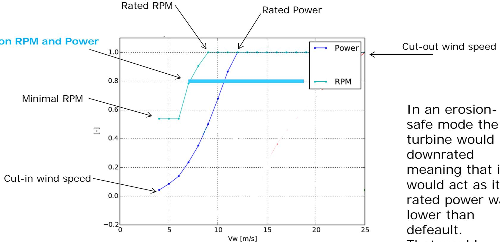
In an erosion-safe mode the turbine would be downrated meaning that it would act as its rated power was lower than default. That would effectively decrease the rated RPMs.
