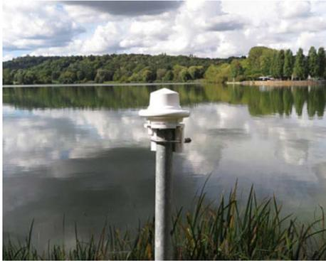
Absolutely maintenance-free and extremely fast measurement of precipitation type (Rain, snow, sleet, freezing rain, hail) and intensity, thanks to radar measurement technology.
